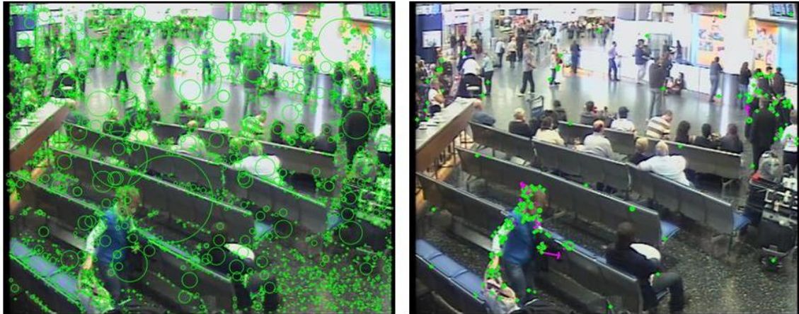
Figure 3.1: Interest points detected with SIFT (left) and MoSIFT (right). Green circles denote interest points at different scales while magenta arrows illustrate optical flows. Note that MoSIFT identifies distinctive regions that exhibit significant motion, which corresponds well to human activity while SIFT fires strongly on the cluttered background.
