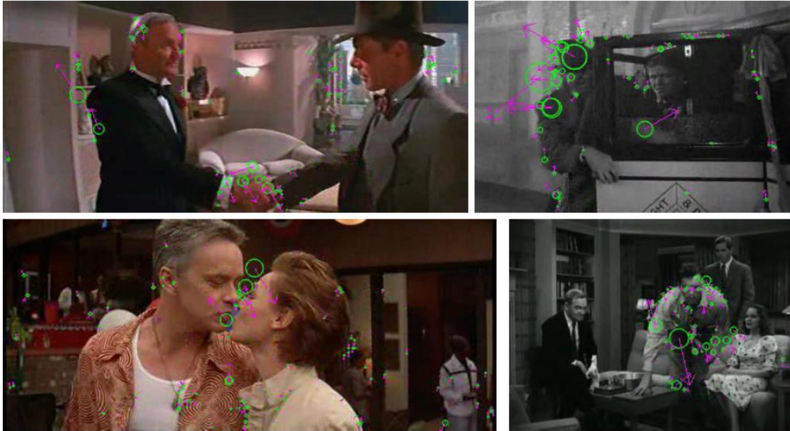
Figure 3.9: Some examples of MoSIFT from the Hollywood dataset. Top left is a handshaking activity. Top right is a man getting out from a car. Bottom left is a kissing activity and a standing up activity in bottom right. A green circle indicates interest points and the purple arrows show the direction of motion.
