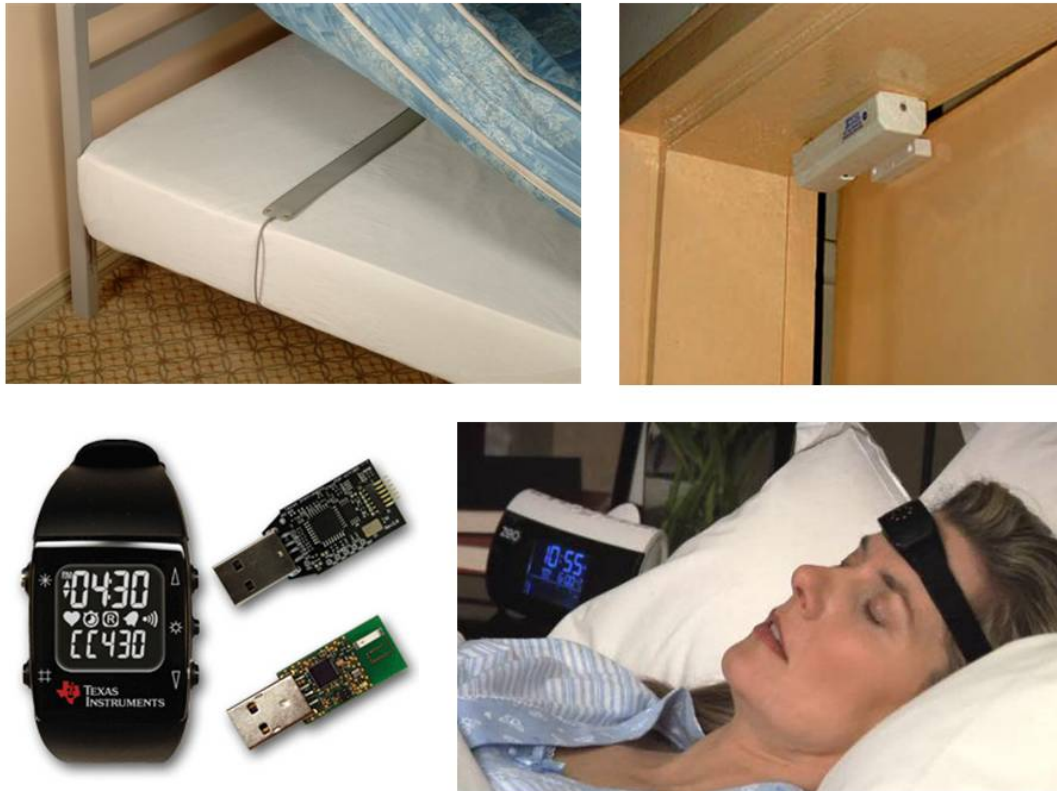
Figure 6.1: Several health care aided device examples. Top left one is a sensor attached to a bed to detect sleeping posture. Top right is a binary sensor to detect door status. Bottom left is a accelerometer in a watch to measure motor activities. Bottom right is a head band which collects brain waves to aid health care (sleeping quality).
