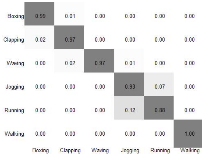
Figure 3.8: Confusion matrix for the KTH activities. This is achieved by 900 video codewords. The major confusions occur between jogging and running.
