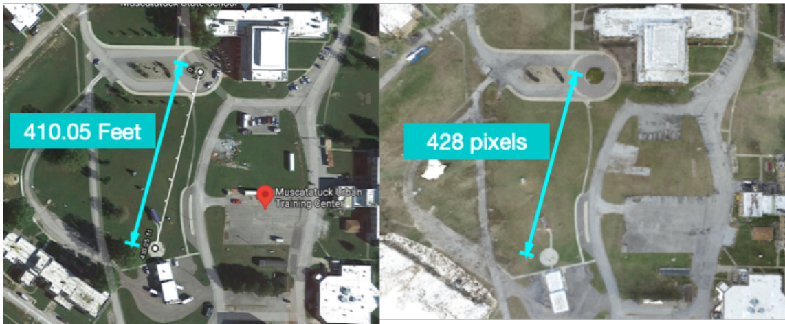
Figure 8.8: MEVA-Trajectory dataset's unit is in feet. On the left is a screenshot of the satellite view of the dataset location, Muscatatuck Urban Training Center, and on the right is the top-down view of the 3D point cloud.
