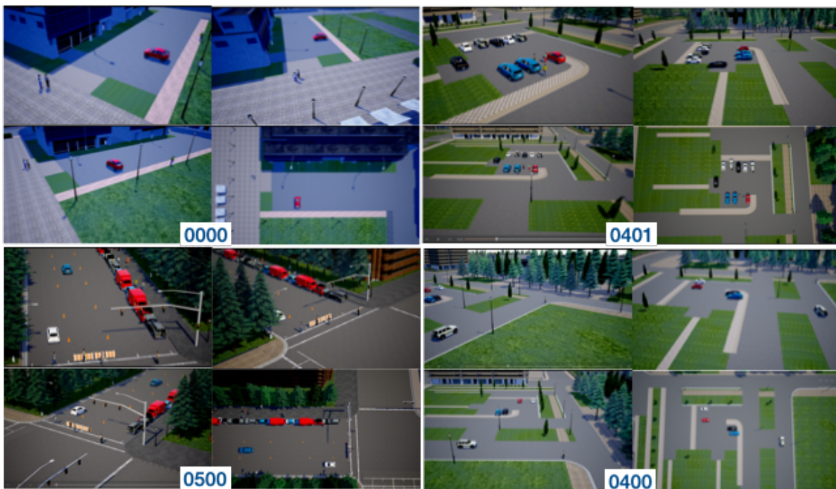
Figure 6.3: Visualization of the multi-view 3D simulation data used in SimAug training. Data generation process is described in Section 6.3.2. We use 4 camera views from 4 scenes defined in [132]. “0400” and “0401” scene have overlapping views. The top-left views are the original views from VIRAT/ActEV dataset.
