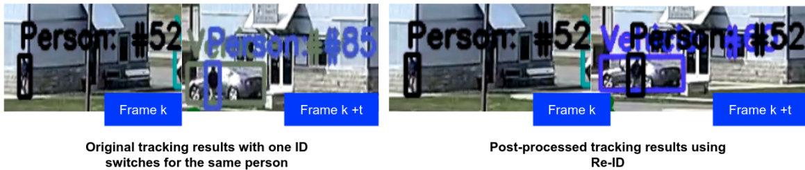
Figure 8.2: Single video object detection and tracking with re-identification. On the left is the original tracking results and on the right is after re-identification. See text for details.
